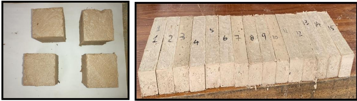
Figure 5 Prepared cubes (on left) and prisms (on right)
